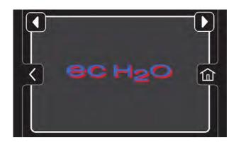
**Yellow ec-H2O Fault Screen** - Machine detected an ec-H2O system water or plumbing fault.
