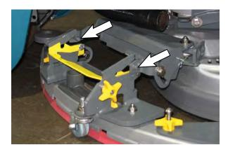
Slide the squeegee assembly onto the squeegee carriage until both squeegee carriage pins are secured in the bracket.
