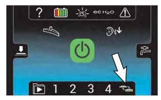
NOTE: Remain standing on the operator presence pedal until the scrub head has moved through the entire range of motion and has stopped moving. Process will be paused if the operator presence pedal is released. Step back onto the operator presence pedal and press brush change button again to continue the process. Turn key switch to OFF position to abort process.
