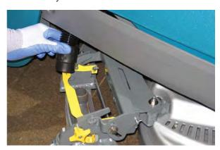
4. Squeeze the squeegee retainer lever and remove the squeegee assembly from the machine.
