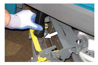
7. Rotate and center the squeegee assembly underneath the machine.
