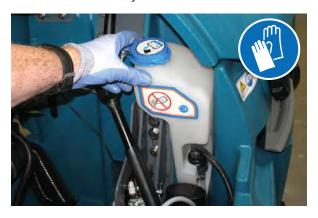
3. Remove the blue cap from the automatic battery watering tank.
