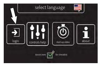
3. First time use - Enter the factory-assigned supervisor mode login code "1234" then press the green enter button.
