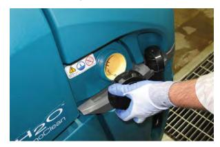
Insert the fill hose into the yellow strainer and ensure the hose is held securely into place in the strainer.
