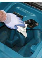
FOR SAFETY: When servicing machine, do not power spray or hose off machine. Electrical malfunction may occur. Use damp cloth.
