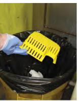
7. Remove and clean the float shut-off screen.
