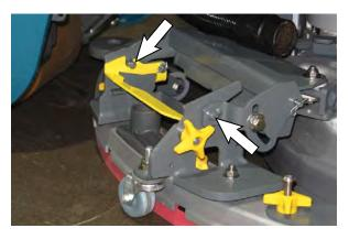
5. Machines with 20 in. (500 mm) scrub heads only: Be sure both squeegee tabs are positioned above the scrub head skirt.
