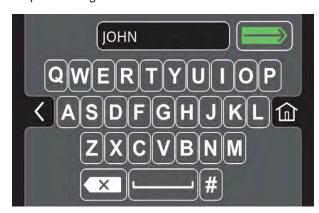
5. Assign a login code for the new user profile then press the green enter button. The new login code can be any combination of numbers ranging from 3 to 8 digits in length.
