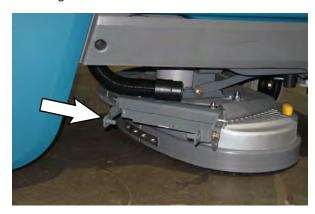
3. Align the squeegee carriage pins into the squeegee assembly bracket.
