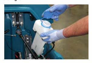
The automatic battery watering indicator will also alert user to add distilled water when tank is empty. See CONTROL PANEL OPERATION for further details.
