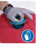
3. Machines with magnetic brushes or pad drivers: Position the brush under the scrub head and lift the brush up onto the scrub head until the magnet in the scrub head secures the brush.
