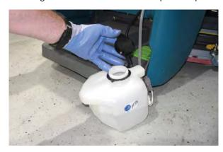
Automatic battery watering option - Refill tank with distilled water. Replace cap.
