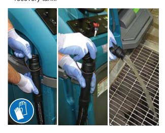
NOTE: When using a bucket to drain the machine, do not use the same bucket to fill the solution tank.
