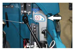
2. Reposition the automatic battery watering tank so that it can be easily filled.
