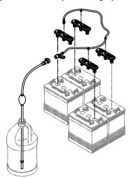
The optional HydroLink battery watering system provides a safe and easy way to maintain the proper electrolyte levels in your batteries. It is designed exclusively for Trojan flooded (wet) lead-acid batteries.
