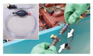
4. Submerge the other end of the hand pump hose into a bottle of distilled water
