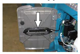
For models equipped with off-board chargers, first connect the charger's DC cord into the machine's battery charge receptacle then plug the AC power supply cord into a properly grounded wall outlet. Refer to the off-board battery charger's owner manual for operating instructions. Do not close the recovery tank on the charger cables when charging with an off-board charger.
