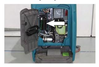
Disconnect the two hose connectors from the top of the cartridge by pressing the gray collars inward and pulling the connectors outward. Lift cartridge to remove.
