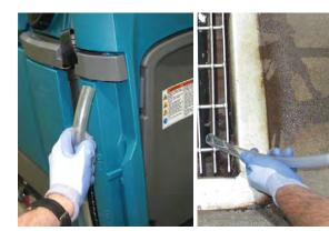
9. Severe Environment option - Refill the Severe Environment tank with a recommended cleaning detergent at full concentration. Replace cap.
