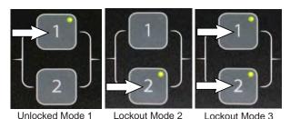
4. Press the solution flow button to configure the zone control button presets for lockout modes 2 or 3.
