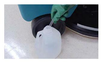
5. Squeeze the bulb on the hand pump hose until firm The white level indicators will raise to the full position.
