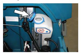
4. Pour distilled water into tank. To avoid getting water on sensitive components, use a funnel to fill automatic battery watering tank.
