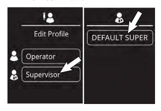
5. Press the factory-assigned login code and enter a new login code. Press the flashing save button to save the new login code.
