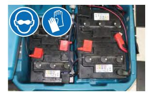
Check the water level in the automatic watering tank periodically. Add distilled water when low.
