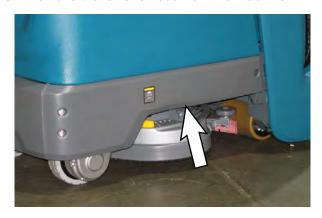
Position a floor jack under the tie down / jack point and arrange all hoses / cables so they are not crushed when the machine is jacked up off the floor.
