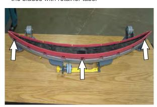
8. Squeeze the squeegee frame and blade retainer together and re-tighten the two outside knobs.
