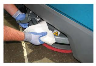
5. Drain, rinse out, and clean the recovery tank. See DRAINING TANKS
