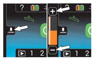
NOTE: If brush pressure is set too high for scrubbing conditions, the brush pressure setting will automatically reduce to a lower setting and begin flashing. When flashing, reduce brush pressure to prevent brush motor overload.
