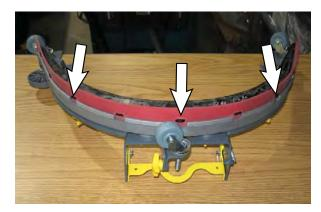
8. Squeeze the squeegee frame and blade retainer together and re-tighten the four knobs.
