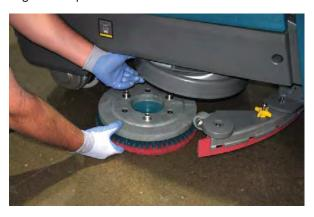
4. Machines equipped with magnetic brush hubs: Push the new brush or pad driver under the scrub head and lift the brush or pad driver until the magnet secures the brush or pad to the drive hub.
