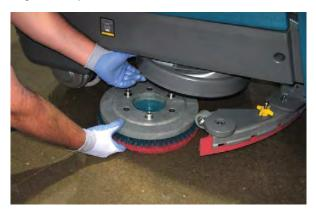
6. Machines equipped with magnetic brush hubs: Push the new brush or pad driver under the scrub head and lift the brush or pad driver until the magnet secures the brush or pad to the drive hub.
