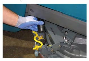
4. Squeeze the squeegee retainer lever and remove the squeegee assembly from the machine.
