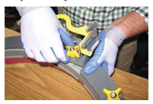
Position the squeegee assembly bracket near the squeegee carriage and align the squeegee carriage pins into the squeegee assembly bracket.
