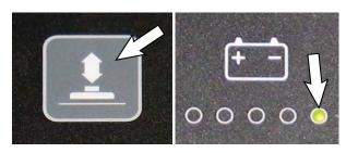
To select or change a supervisor control mode, press and hold the specific zone control button until the LED blinks three times. For lockout mode 3, press and hold zone control buttons 1 and 2 at same time. After selection is made, the LED will turn solid to indicate new mode.
