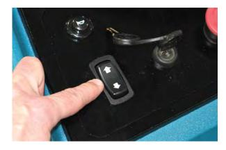
NOTE: If forward / reverse switch lights are flashing rapidly, be sure right foot is not pressing the green go pedal. The machine will not accept input from the forward / reverse switch if the lights are rapidly flashing.
