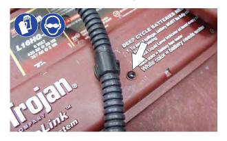
3. Locate the battery fill hose coupler inside the battery compartment. Remove the dust cap and connect the hand pump hose.
