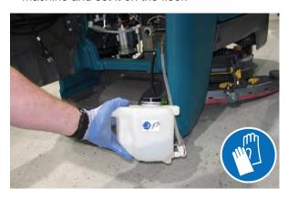
NOTE: Remove the Severe Environment tank from the machine before filling the tank with detergent to prevent damaging electronic components.
