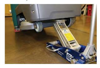
5. Place a jack stand underneath the other jack point and lower the machine onto the jack stand so both the jack stand and floor jack are supporting the weight of the machine.
