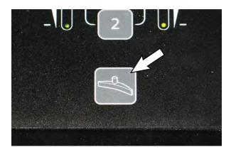
Machines equipped with Pro-Panel: Press the 1-Step button and then the vacuum fan button. The vacuum fan button will no longer be illuminated and the vacuum fan will stop operating.
