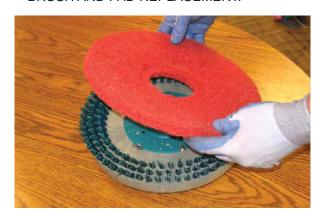
Replace brushes when they no longer clean effective. See BRUSH AND PAD REPLACEMENT. Wipe the squeegee blades clean. Inspect blades for wear and damage. Rotate blades if worn. See SQUEEGEE BLADE REPLACEMENT.
