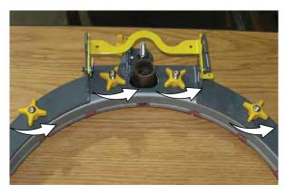
6. Remove worn blade(s) from the blade retainer.
