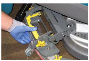
5. Fully loosen the two outside knobs on squeegee assembly. This will separate the spring loaded blade retainer from squeegee frame.
