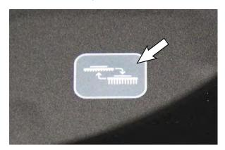
Machines with magnetic brushes: Press the brush change button to release the brush(es) from the scrub head. The scrub head will completely raise to disengage the brush(es) from the scrub head, and then partially lower to allow the brush(es) to be removed from under the scrub head. Reinstall brush(es) with scrub head in partially lowered position.
