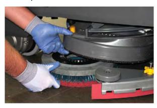
Machines with 3-lug brush hubs: Position the three lugs into the motor hub slots and give the pad driver / brush a quick counter-clockwise turn to engage hub.
