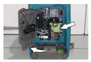
2. Remove the Severe Environment tank from the machine and set it on the floor.
