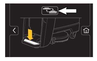
The brush change button will turn green while the scrub head repositions to allow the brush or pad driver to be changed.
