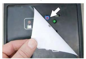
Using a small standard screwdriver, turn the dial to the appropriate battery type according to the following chart.
