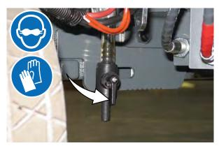
Close the battery compartment drain valve after all liquid has drained from the battery compartment.
