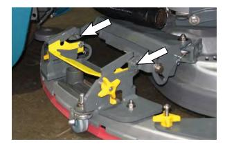
Slide the squeegee assembly onto the squeegee carriage until both squeegee carriage pins are secured in the bracket.
