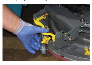
5. Fully loosen the four knobs on squeegee assembly. This will separate the spring loaded blade retainer from squeegee frame.
