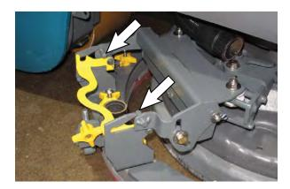
10. Slide the squeegee assembly onto the squeegee carriage until both squeegee carriage pins are secured in the bracket.
