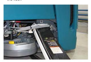
5. Use a floor jack to raise machine from the floor.
