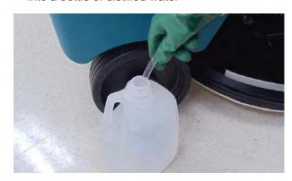
Squeeze the bulb on the hand pump hose until firm. The level indicators will turn black when full.
