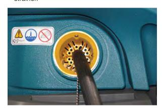
Fill the solution tank with water until level reaches the 53 L (14 G) mark on the solution tank indicator.
