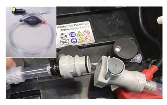
Submerge the other end of the hand pump hose into a bottle of distilled water.
