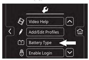
Select battery type and brand installed in machine. See battery label to determine type and brand. Press the up and down arrows to scroll through battery selection.
