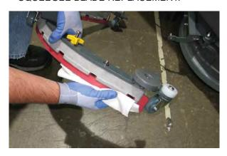
4. Clean scrub head skirt. Check for wear and damage. Replace if worn or damaged.
