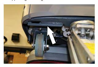
When finished with maintenance, use floor jack to raise machine from jack stand, remove the jack stand from under the machine, and lower the machine to the floor.
