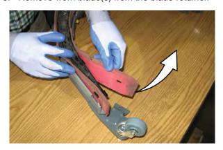
7. Rotate the rear blade(s) to a new wiping edge and reinstall blade(s). Make sure to align the slots in the blade(s) with retainer tabs.
