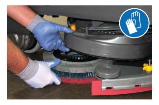
Machines equipped with 3-lug brush hubs: To remove the brush or pad driver, grip the disk and give it a quick turn.
