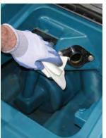
FOR SAFETY: When servicing machine, do not power spray or hose off machine. Electrical malfunction may occur. Use damp cloth.
