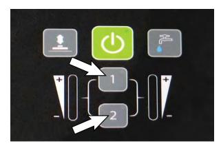
To preset the zone control buttons for different scrubbing applications, select the desired settings from list below, then press and hold the zone button until the green LED blinks three times to save preset. To preset zone 3, press and hold zone buttons 1 & 2 at the same time.
