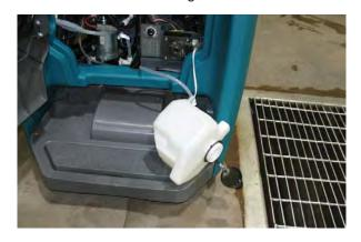
Models not equipped with ec-H2O system - Turn machine on and operate the solution flow system. Turn the machine off when the antifreeze is visible on the floor.
