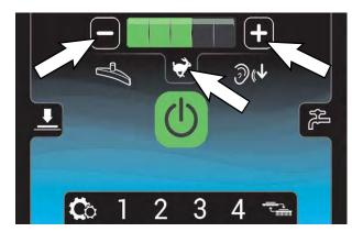
4. Press the (+) button to increase the maximum scrub speed. Press the (-) button to decrease the maximum scrub speed.
