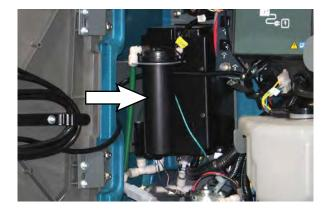
The control panel will signal the following code when it's time to replace the cartridge. The ec-H2O icon will begin to blink blue and red. See SERVICE INDICATOR CODES for further details.
