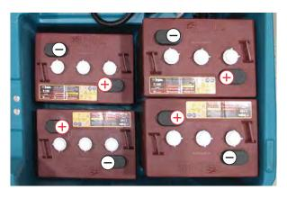
Using the supplied battery post boots, connect the cables to battery posts, RED TO POSITIVE (+) & BLACK TO NEGATIVE (-). Tighten cable connections to batteries per battery manufacturer specifications.
