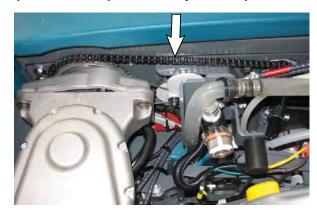
Check the steering cable for damage or wear.
