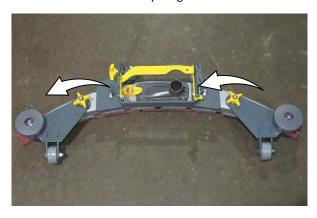
6. Remove worn blade(s) from the blade retainer.
