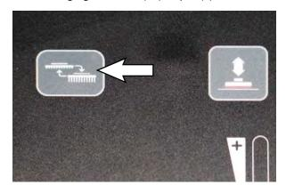
NOTE: Remain standing on the operator presence pedal until the scrub head has moved through the entire range of motion. Process will be paused if the operating presence pedal is released. Step back onto the operator presence pedal and press the brush change button again to continue the process. Turn key switch to OFF position to abort process.
