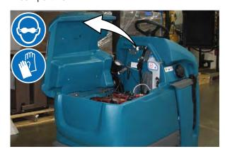
2. Carefully install the batteries into the battery compartment tray and arrange the battery posts as shown.
